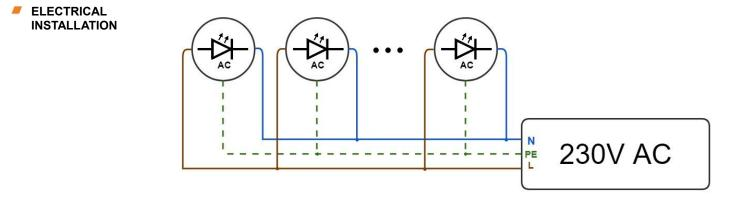
Connecting to the power supply should be done when the power supply is off.
